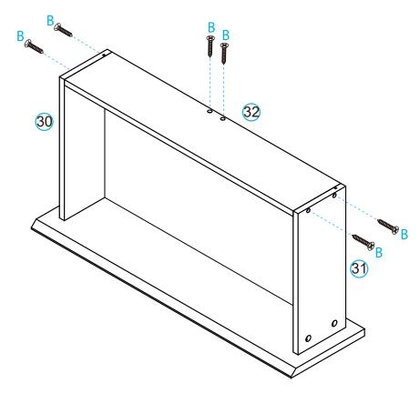
Attach panels [30] and [31] to panel [32] secure with 4x screws (B) and panel [32] to panel [34] secure with 2x screws (B). Tighten with a screwdriver.
