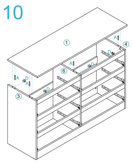
Attach panel [1] to panels [3], [4] and [6] with 6x dowels (A) and secure with 6x locking nuts (D). Tighten with a screwdriver.
