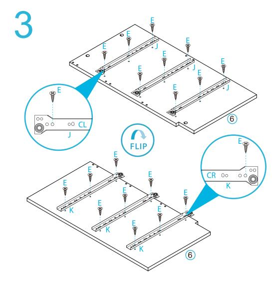
Attach 3x slide rails (J) and 3x slide rails (K) to panel [6] as shwon. secure with 18x screws (E). Tighten with a screwdriver.
