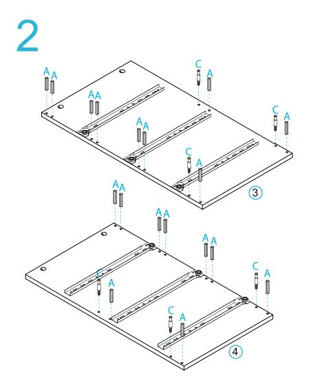
Insert 18 x dowels (A) into panels [3] and [4]. Attach 6 x bolts (C) into Panels [3] and [4] as shown. Tighten with a screwdriver.
