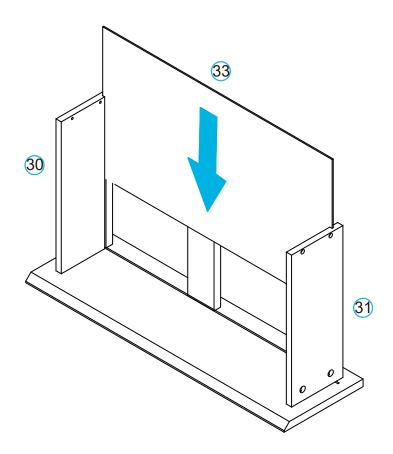
Slide panel [33] down along the grooves between the panels [30] and [31] as shown.
