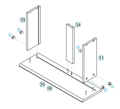
Attach panels [30], [31] and [34] to panels [35]/[36] secure with 5x locking nuts (D). Tighten with a screwdriver.
