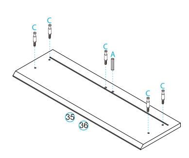
Insert 5x bolts (C) and 1x dowel (A) into panels [35]/[36]. Tighten with a screwdriver.
