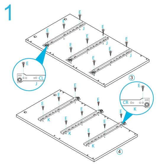
Attach 3x slide rails (J) to panel [3] and secure with 9x screws (E). Tighten with a screwdriver. Attach 3x slide rails (K) to panel [4] and secure with 9x screws (E). Tighten with a screwdriver.
