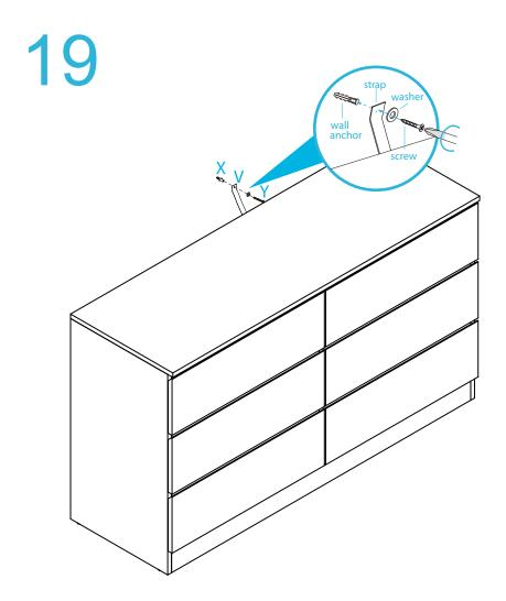
Once assembled lift furniture into place, do not drag. Use a drill to create a small hole lining up with the top of the safety strap (V). Fasten to the wall using 1x washer (Z), 1x wall anchor (X) and 1x wall screw (Y). Ensure unit is balanced and steady before use. You're done, enjoy!
