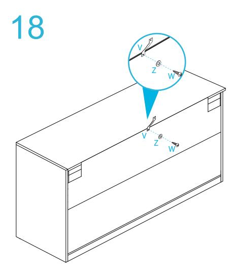
Attach 1x safety strap (V) to the top of the back side of the unit as shown using 1x washer (Z) and 1x screw (W). Tighten with a screwdriver.
