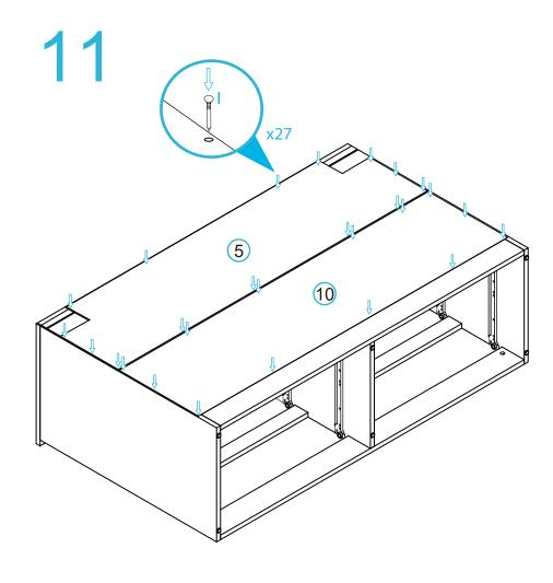
Attach both back panels [5] and [10] to the cabinet using 27x nails (I) and using a hammer.
